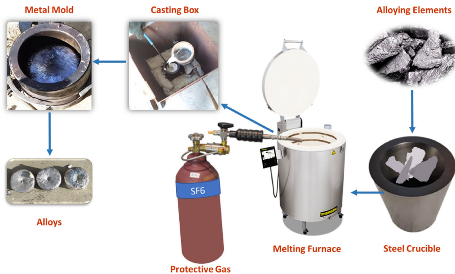
Figure 1. Schematic illustration of the casting process.
