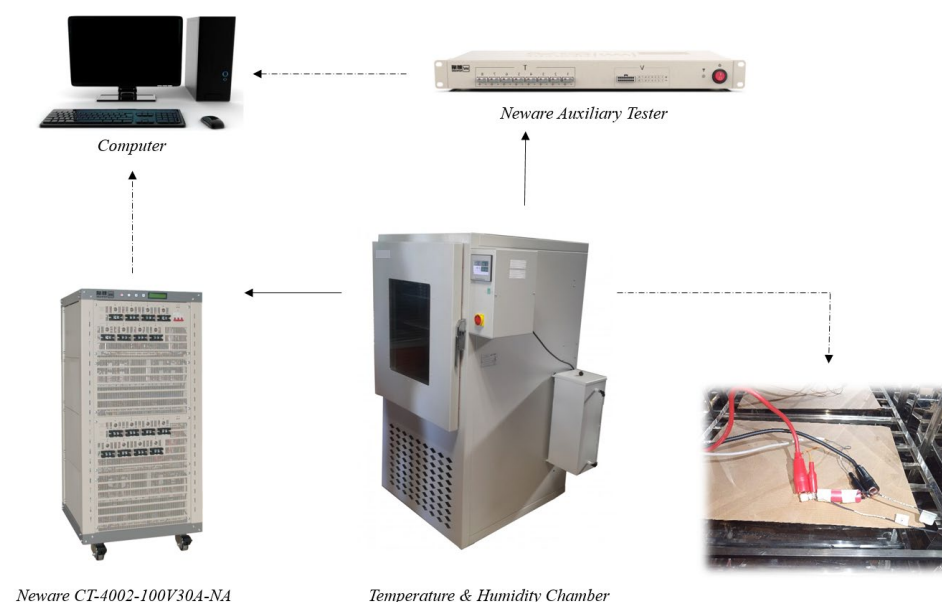
Figure 1. Battery charge and discharge experimental system.
