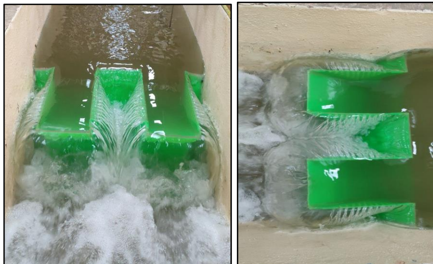
Figure 4.10: The flow across inlet and outlet key of PKW by adding screen wall with holes to it at high head of flow ( H_1/P > 0.2 ).
