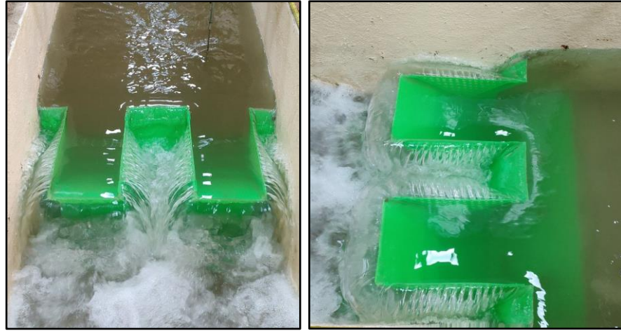
Figure 4.12: The flow across inlet and outlet key of PKW by adding screen wall with holes to it at head of flow much higher than ( H_1/P > 0.2 ).
