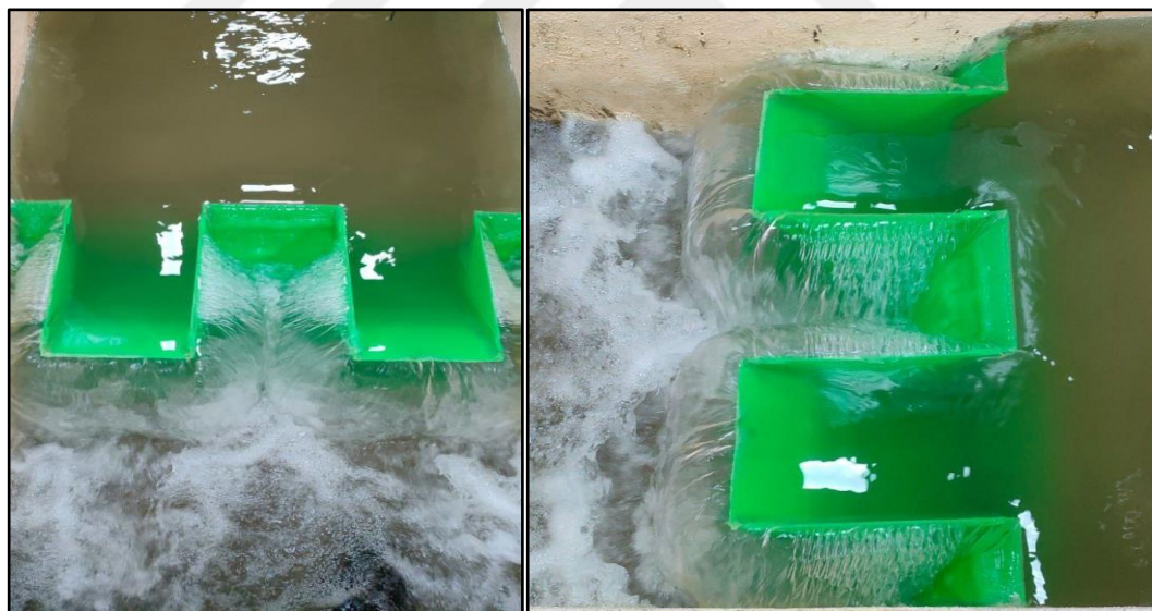
Figure 4.6: The flow across inlet and outlet key of PKW by adding screen wall with holes to it at low head of flow ( H_1/P < 0.2 ).
