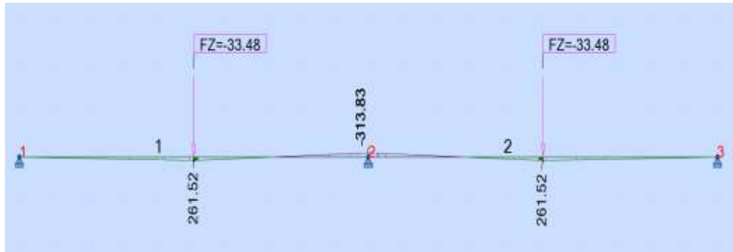
Figure A.29: KEL Bending Moment Per Girder
