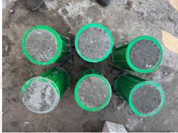
Figure 4.35: Compressive Strength Test
