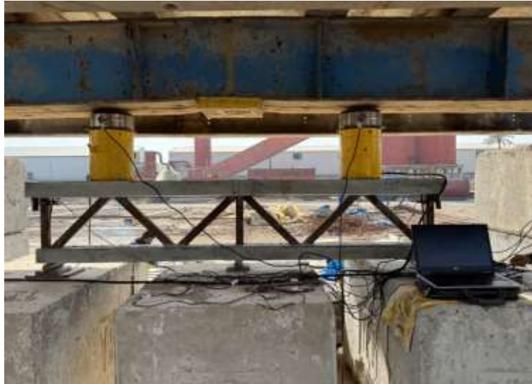
Figure 4.47: Load Operation Setup In Universal Hydraulic Machine for Category Two (DCTG)
