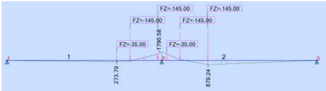
Figure A.10: Bending Moment Due to HL-93 Truck Live Load at Mid Support
