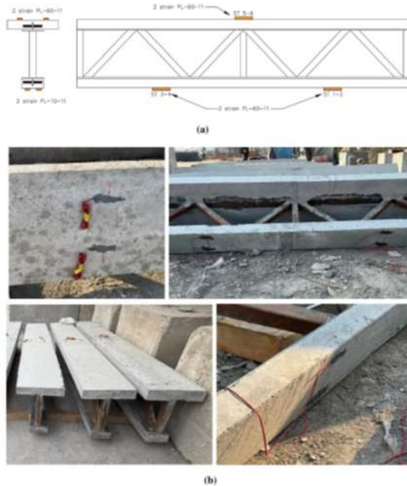
Figure 4.38: Position of the Strain Gauges for Category One Specimens (DCTG). (a) Strain Gauge Location Drawing Sheet for the (DCTG), (b) Site Installation of the Strain Gauge for the (DCTG)
