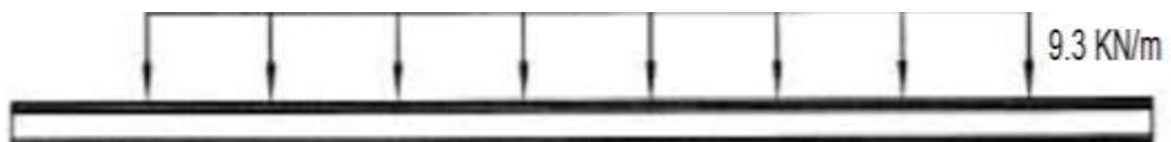
Figure A.19: Typical Design Lane Live load
