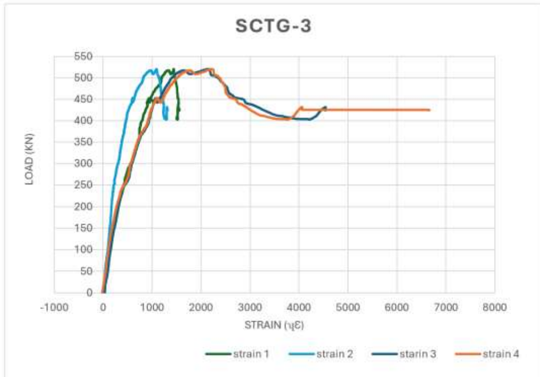
Figure 6.22: Bottom Steel Flange Load – Strain Curve for the SCTG-3
