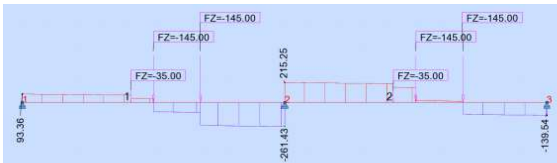
Figure A.8: Reactions Due to HL-93 Truck Live Load at Mid Span
