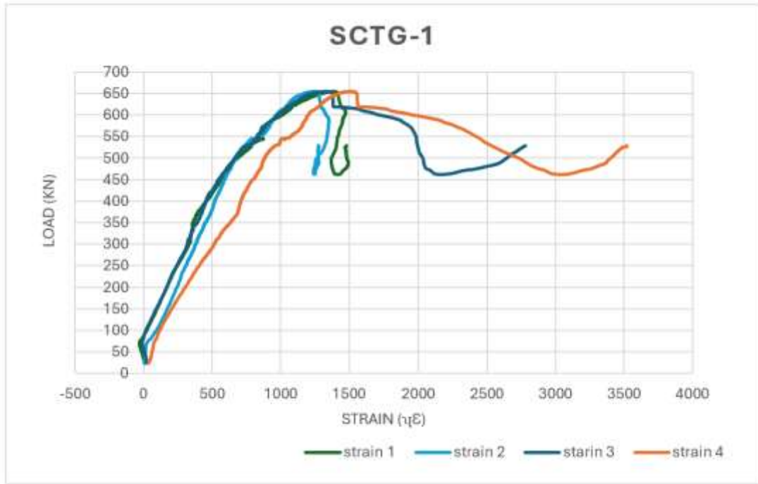
Figure 6.20: Bottom Steel Flange Load – Strain Curve for the SCTG-1
