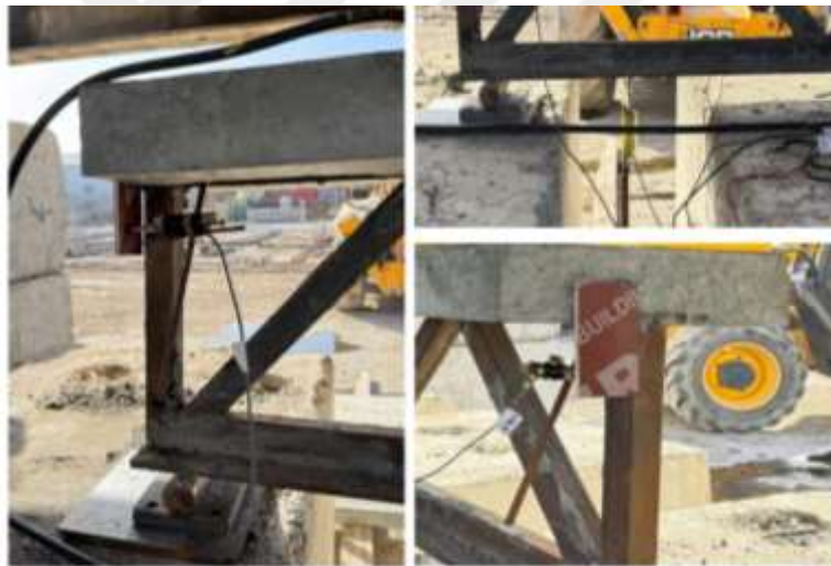
Figure 4.40: Site Installation of the LVDT Indicator for Category One Specimens (SCTG)
