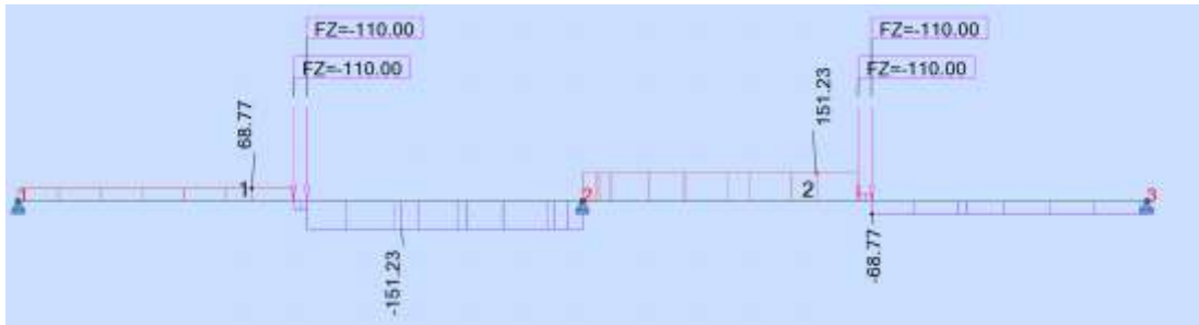
Figure A.15: Shear Force as Tandem Design Live Load at Mid Span
