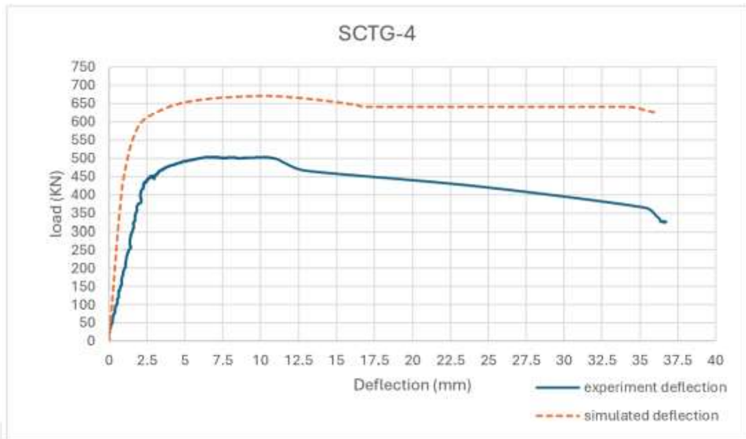
Figure 6.57: Load – Deflection Of Simulate and Experiment Test for the SCTG-4
