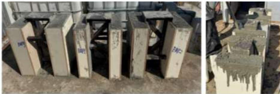
Figure 4.16: Concrete Pouring of the Push-Out Specimens
