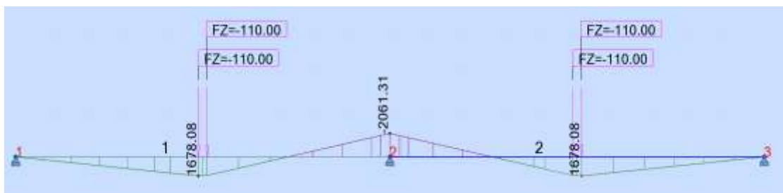
Figure A.14: Bending Moment as Tandem Design Live Load At Mid Span
