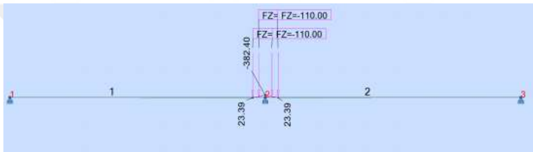
Figure A.17: Bending Moment as Tandem Design Live Load at Support p3
