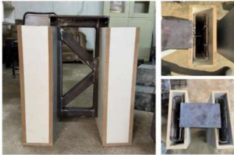
Figure 4.15: Installation of the Wooden Casting Mold with the Samples
