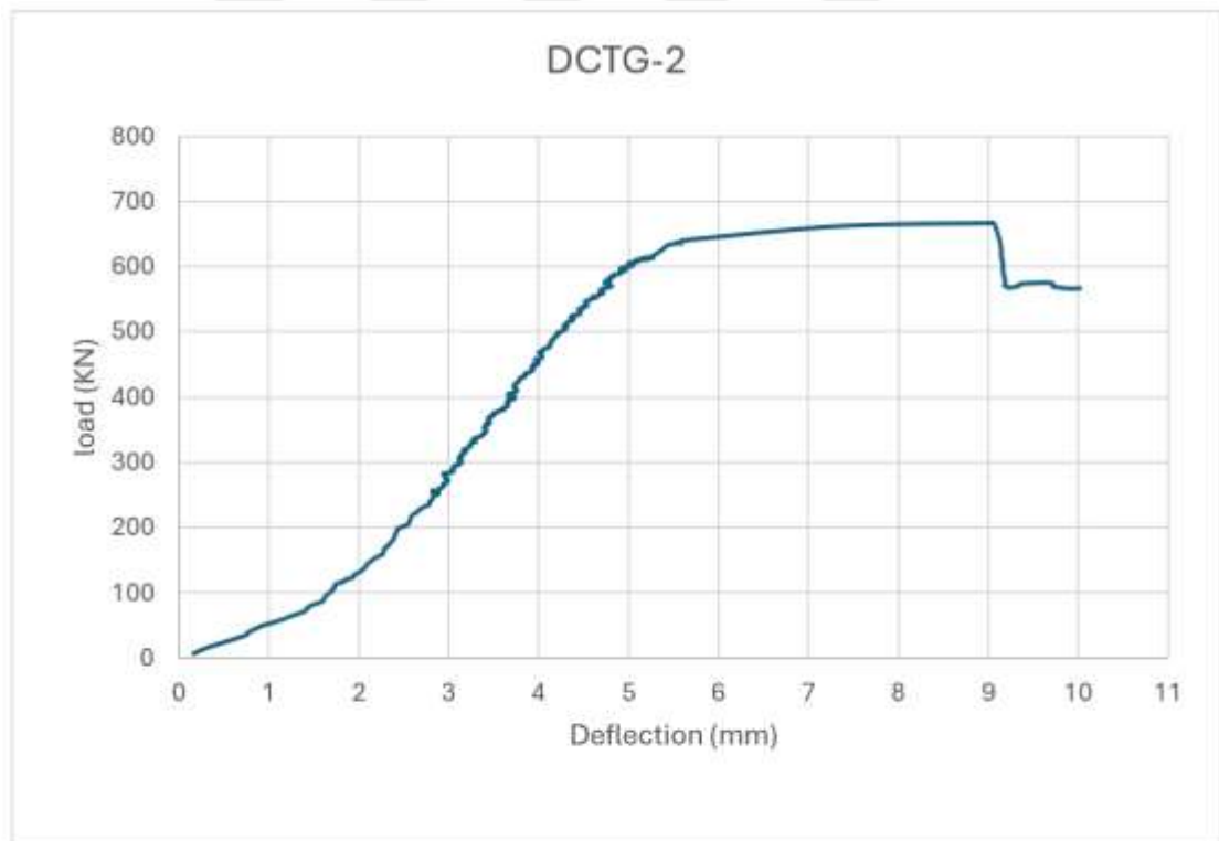
Figure 6.37: Load-Deflection Curve of the DCTG-2
