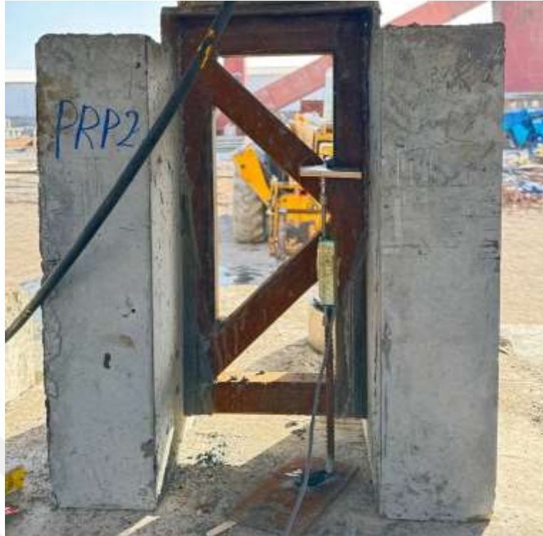
Figure 4.8: Position of LVDT Device for the Push-Out Samples
