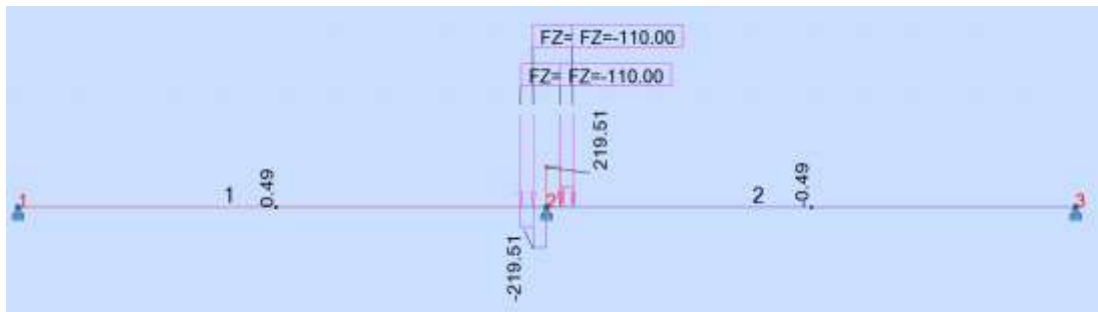
Figure A.18: Shear Force as Tandem Design Live Load at Support p3
