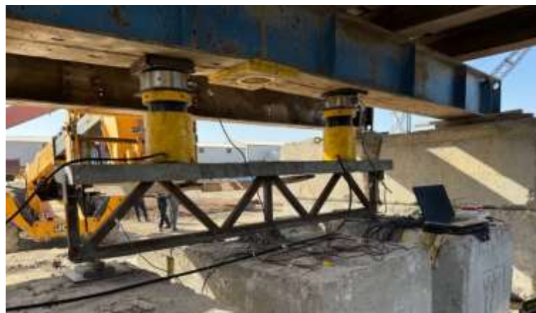
Figure 4.46: Load Operation Setup In Universal Hydraulic Machine for Category One (SCTG)
