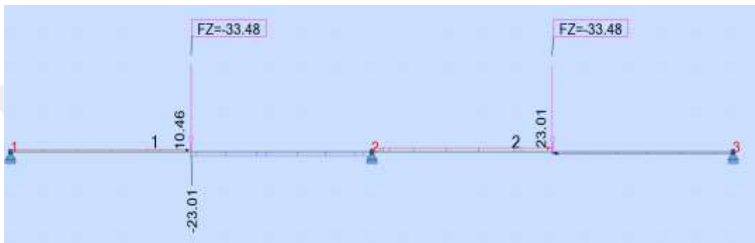
Figure A.30: KEL Shear Force Per Girder
