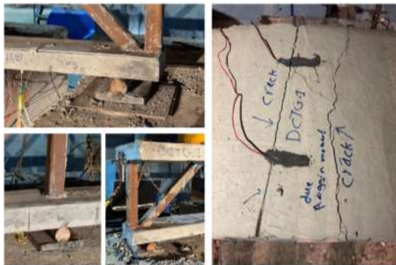
Figure 6.32: Initial and Ultimate Cracks Pattern of the DCTG-1
