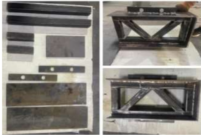
Figure 4.9: Push Out Test Specimens Steel Parts Welding
