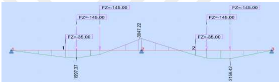
Figure A.7: Bending Moment Due to HL-93 Truck Live load at Mid Span
