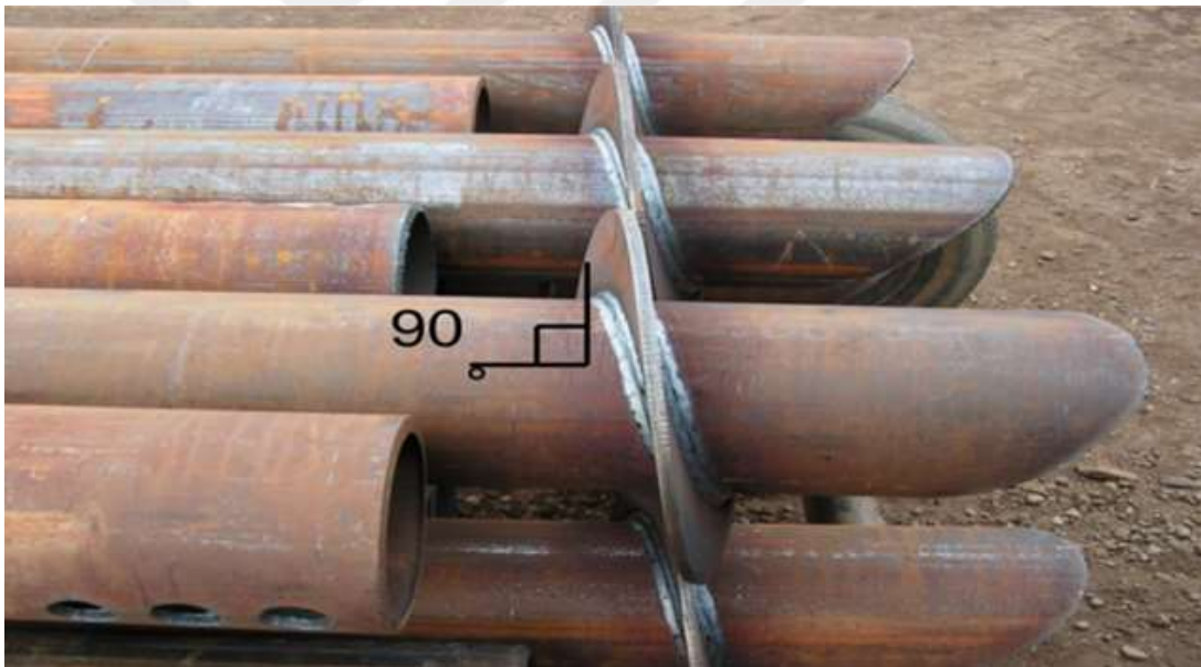
Figure 2.4: Screw Pile with A Shaft-Helix Arrangement
