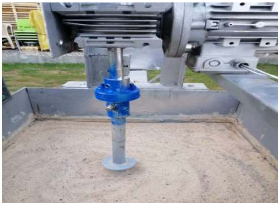
Figure 3.14: Second Gearbox and the Fixating Screw Pile
