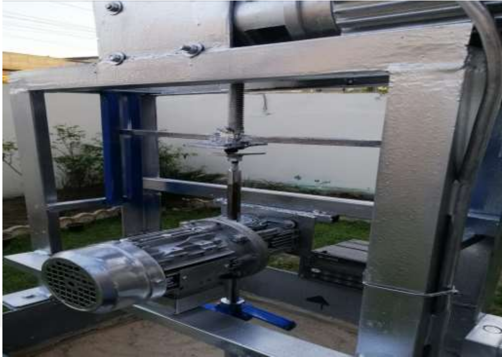
Figure 3.15: The Installation Screw Piles
