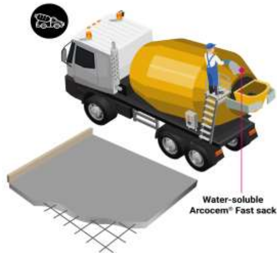
Figure 3.6: Coloring of Concrete
