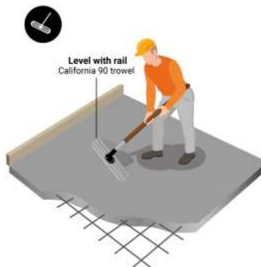
Figure 3.4: Leveling of Concrete
