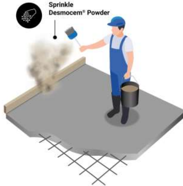
Figure 3.9: Stamped Concrete on the Pavement
