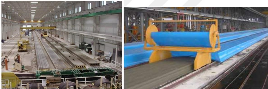
Figure 2.27: Some Stages of Hollow Core Production
