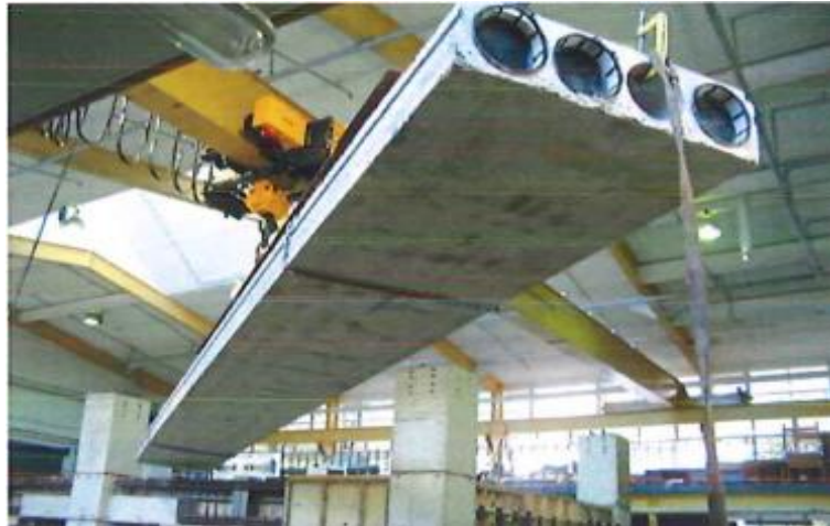
Figure 2.20: Hollow Core Slab System
