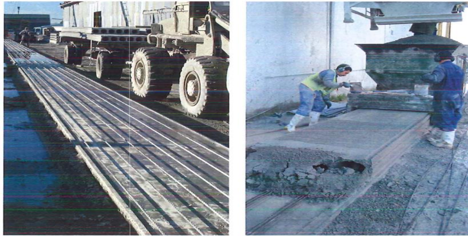
Figure 2.26: Extrusion of a Hollow Core Floor Unit
