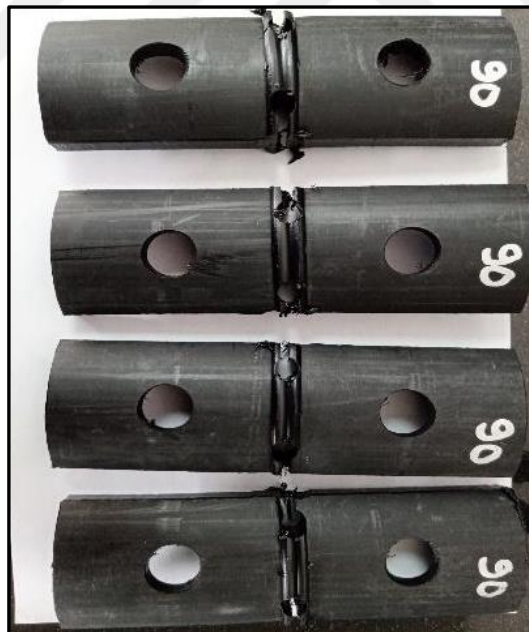
Figure 6.15: The extracted butt fused samples for tensile strength test
