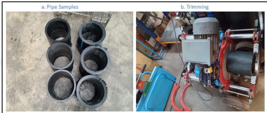
Figure 6.9: The pipe samples (a) and trimming (b)
