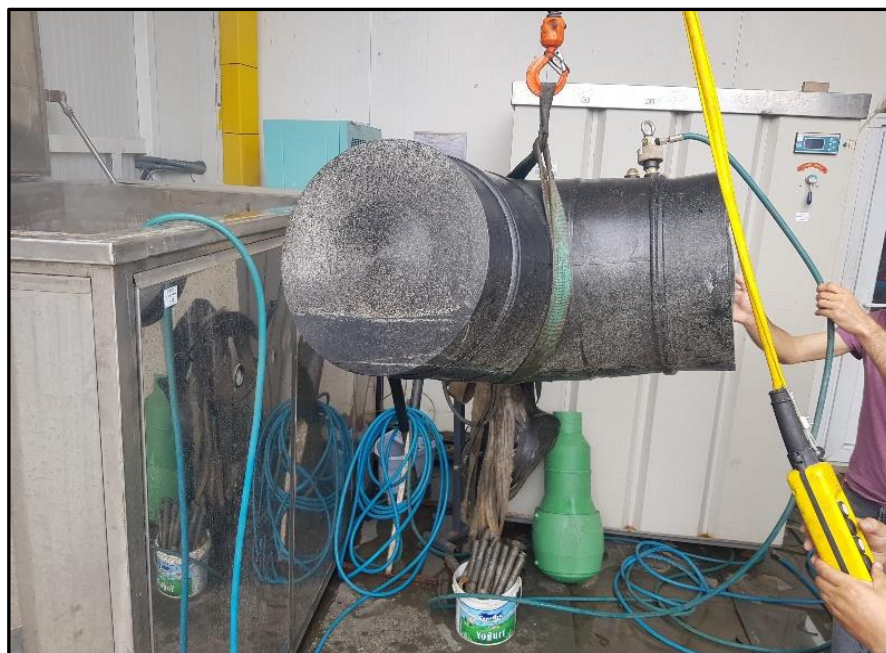
Figure 6.30: The tested samples were removed from the boiler, after visual inspection, no damage was observed
