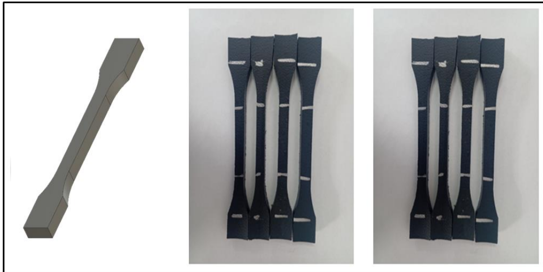
Figure 6.4: Preparation of type 1 test pieces from a 90 mm HDPE Pipe with 8.2 mm wall thickness
