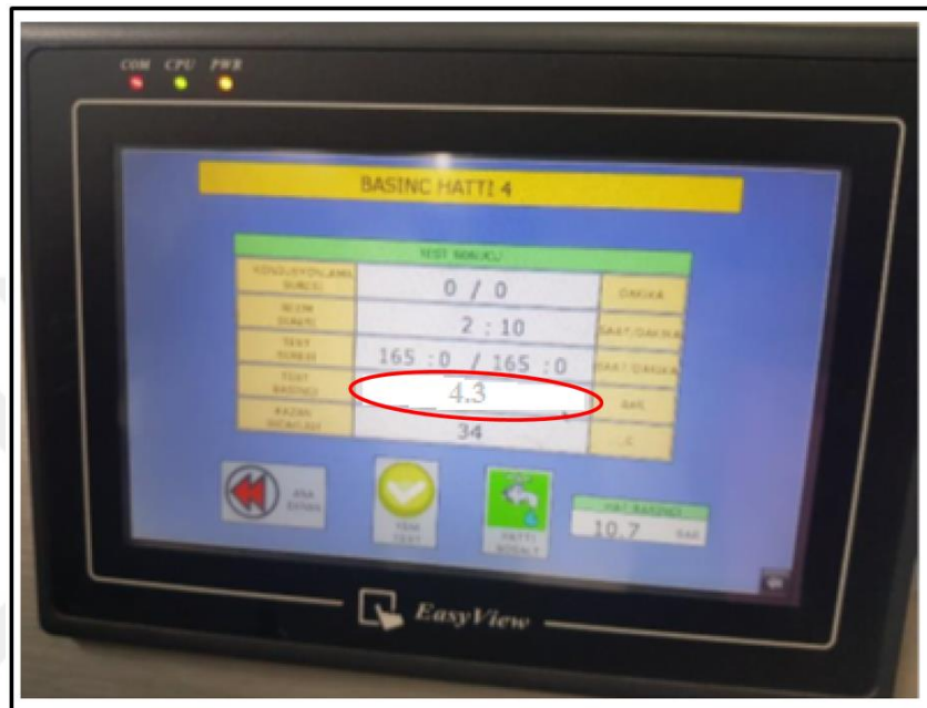
Figure 6.29: Test 165 h / 80 °C / 5,4MPa was successfully completed
