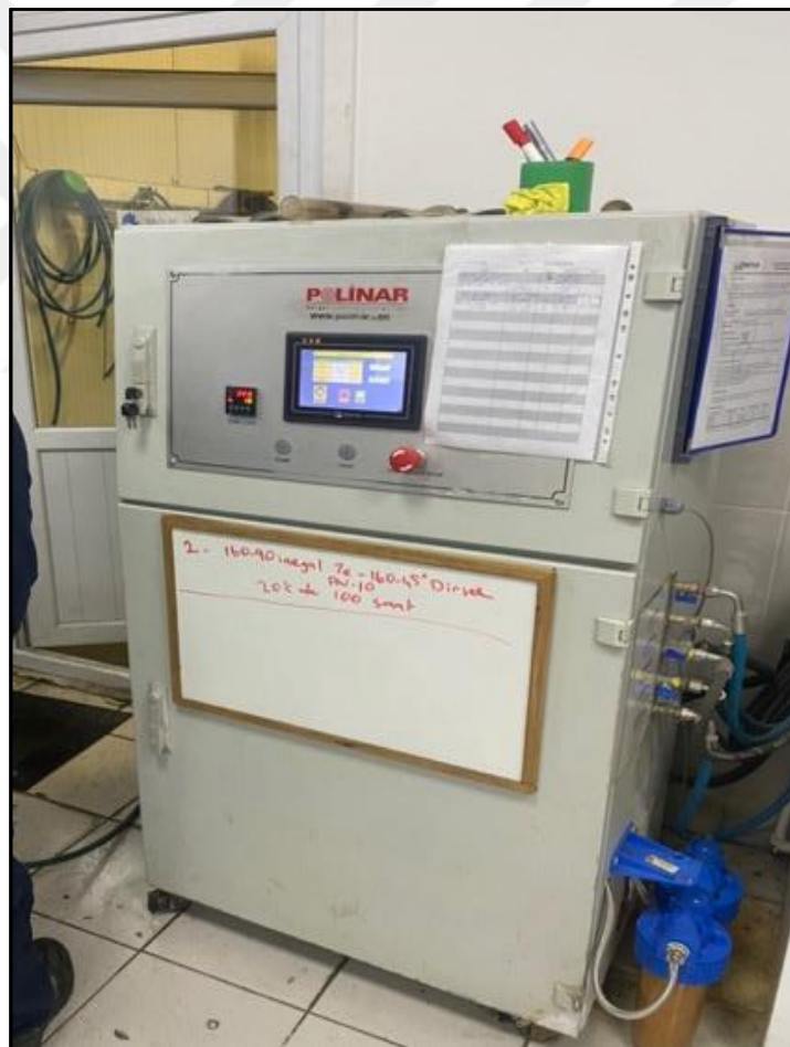
Figure 6.27: The testing equipment for hydrostatic pressure
