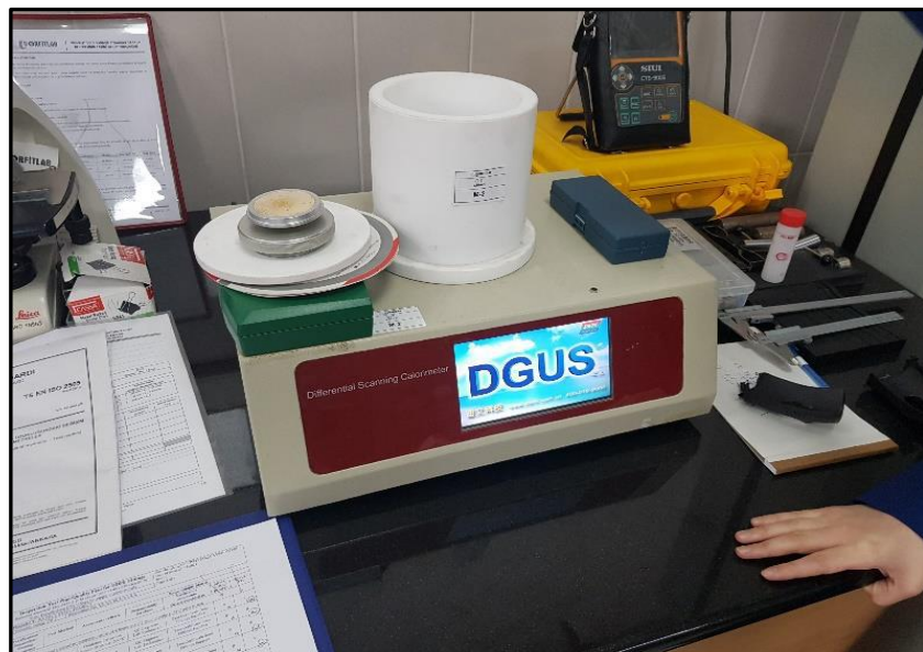
Figure 6.31: The testing equipment for thermal stability
