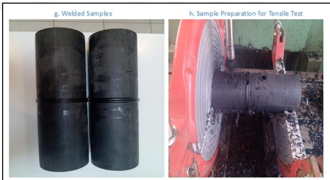
Figure 6.12: The welded samples (g) and machining for tensile test sample extraction (h)
