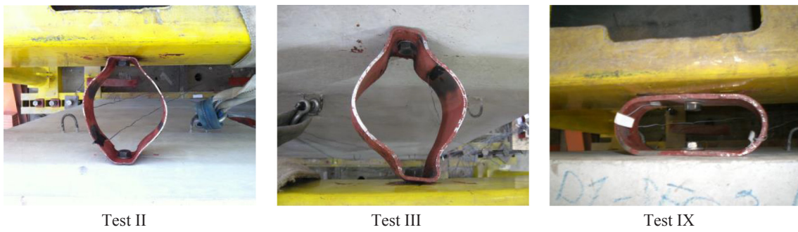
Fig. 25. Deformed shapes of SCs in the PB connection (top view).
