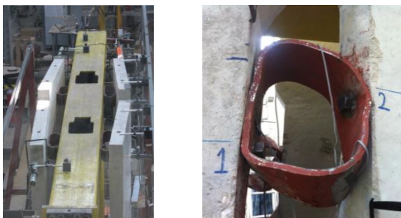
(a) Large out of plane deformations of panels (b) Large deformation of SC at PP connection
