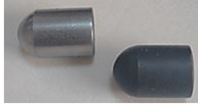
Figure 1. The samples used in the experiments before and after boronizing
