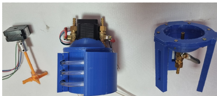
Figure 5. AM-based reactor components (main body with heat exchanger and mixer).
