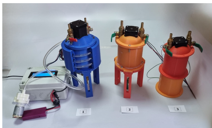
Figure 6. AM-based continuous processing reactor system for the synthesis of metronidazole derivatives.
