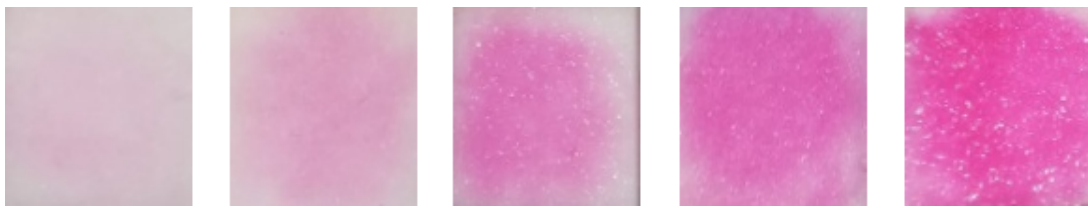
Figure 3.1. Color Scale Resulting from the Reaction of Stock Solutions Containing 4.5, 6.25, 12.5, 25, and 50 \mu\text{L}/\text{mL} Cortisol with the Appropriate Ratios of Color Reagents
