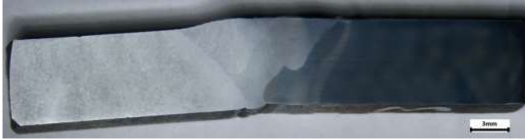
řekil 6.3: P500-WAAM ER110 Makro İnceleme Grnts
