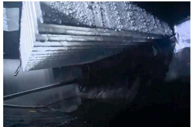
Fig. 10. Condensing water on the cold-side extended surfaces.
