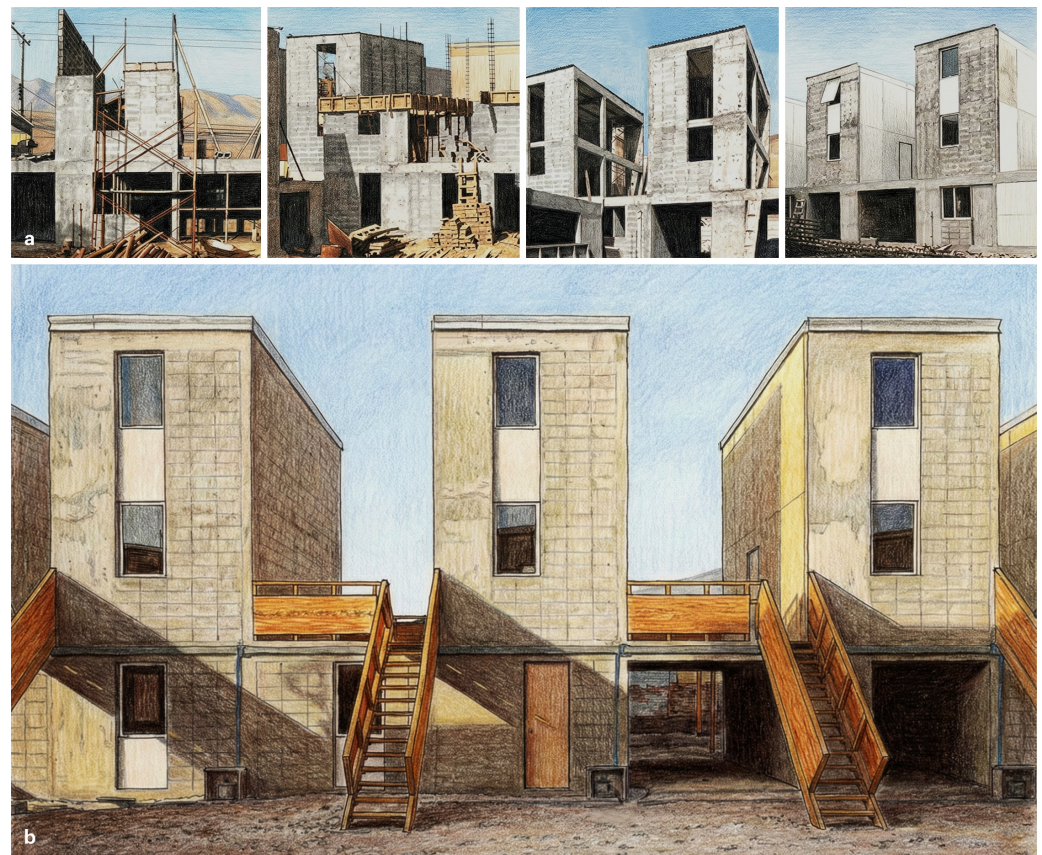
Figure 3. The genesis of the host structure. (a) Construction stage of the fixed structural skeleton encoded by the architect as the DNA [22]. (b) Raw initial state of the Half House delivered to the user before intervention [23]. (Redrawn by the authors based on [22,23]).
