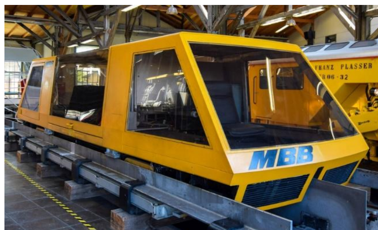
Figure 2.1: Transrapid 01 it Was an Indoor-Only Model Tested On a 6-Meter Long Track With A Top Speed of 48 km/h
