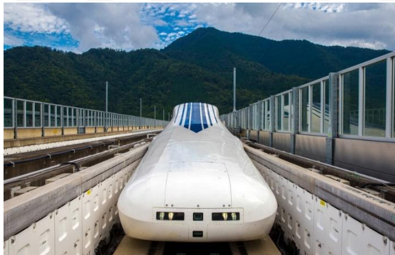
Figure 2.4: L0 Series Shinkansen the fastest maglev with speed up to 603 km/h
