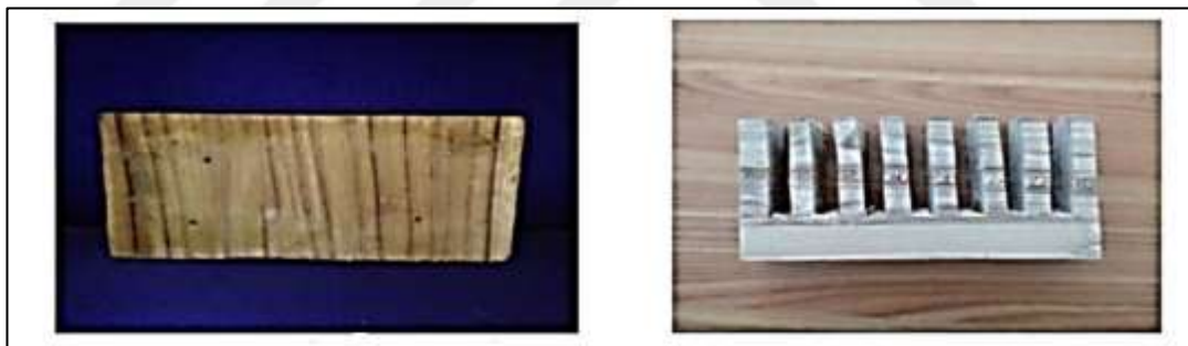
Figure 2.2: The Experimental Model of a Spur Dike That Is both Permeable and Impervious
