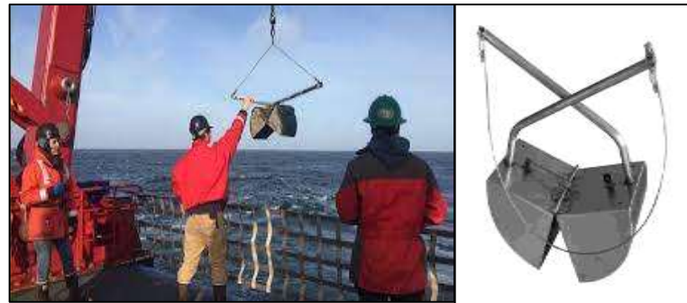
Figure 4.15: Van Veen Grab Device
