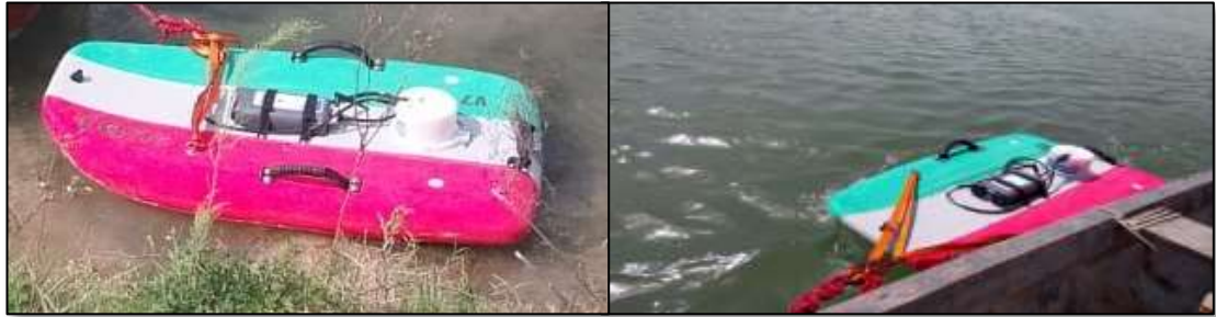
Figure 4.8: The River Surveyor ADCP
